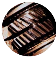
Gearbox damage with evidence of wear
